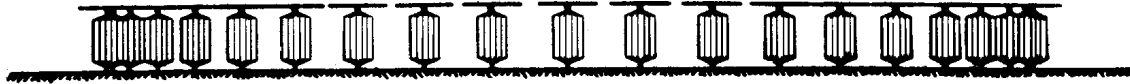
Figure 8: Wullenwever's horizontal view, we can see clearly why sine-law compensation is necessary
