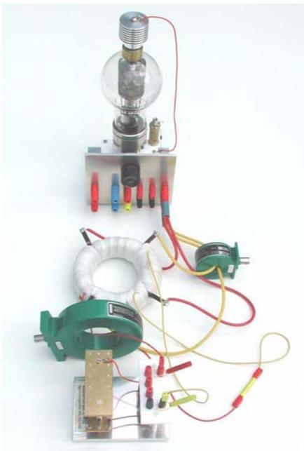
An experimental laboratory setup for the function of the Hohentwiel modulator, with the new pulse transformer. The two green wide-band pulse transformers are used for measurement of the primary and secondary pulse currents. The unit at the bottom with the brass bar is a 1000 ohms non inductive dummy load, simulating the transmitter load. The peak voltage of the high voltage pulse is measured with a Sensitive Research electrostatic crest voltage meter.
